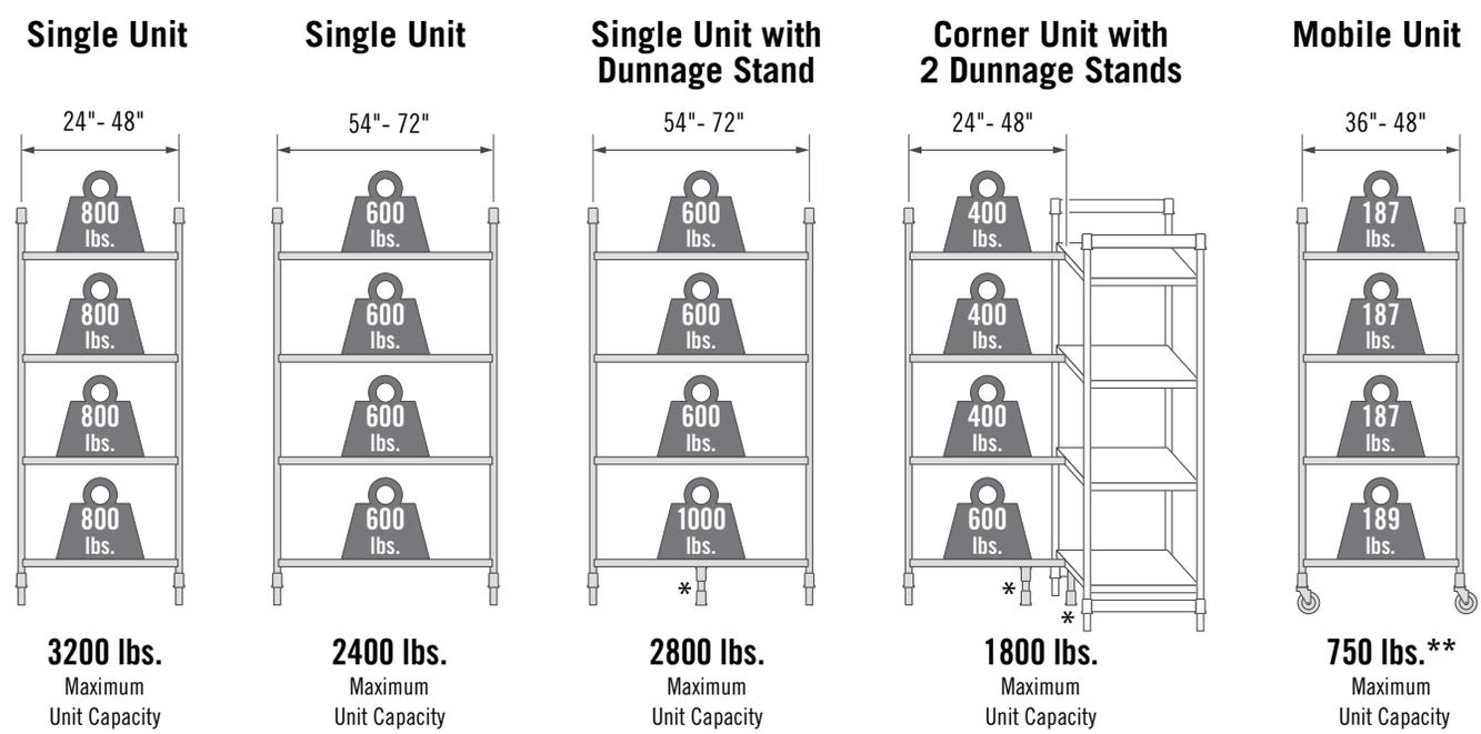
\* Dunnage Stands add stability and increase weight bearing capacity on bottom shelf only. Add to any shelf length. Highly recommended for Starter Units 54" and longer, all Corner Units, U-Shape Units and units specified for heavier loads (See page 10).
