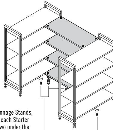
Use four Dunnage Stands, one under each Starter Unit and two under the bottom Intermediate Shelf.
